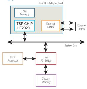
Dual Gigabit HBA Card with LE2020™ TCP/IP Offload Engine
