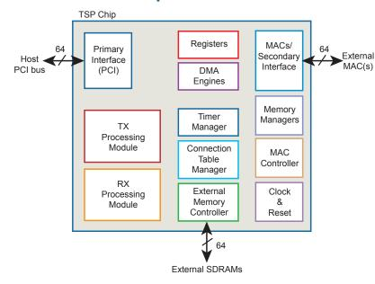
TCP/IP Offload Engine Chip LE2020™
