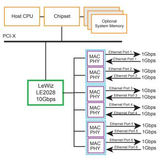
10Gbps Multi-Port TCP/IP Offload Engine
