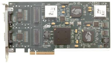
Dual port, 10 GigE, CX-4 Copper/ Fiber Optical NIC, **Dual TOE Engine, PCI-Express**
